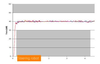
Braking: force step test
