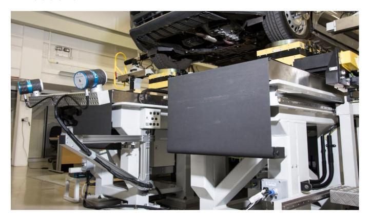
The AB Dynamics K&C Inspect System provides precise measurements of vehicle body and component deflections during vehicle Kinematics and Compliance (K&C) tests on an SPMM 5000e. By integrating vision system measurement technology from AICON into the SPMM control system, the relationship between applied forces and vehicle body and component deflections is precisely captured.
